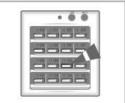
2 To turn on/off a specific air conditioner, press the (ON/OFF) button.
